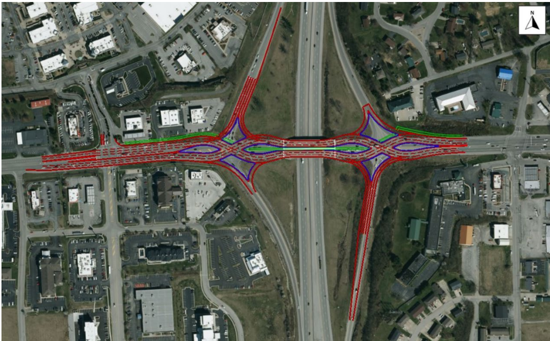
Figure 7: Double Crossover Diamond (DCD) Concept
