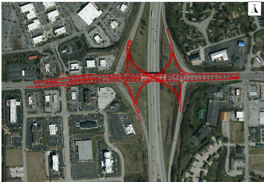
Figure 8: Single-Point Urban Interchange (SPUI) Concept
